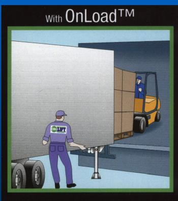
With OnLoad™ delployed, rear end of trailer flush with dock allow forklift on and off freely
