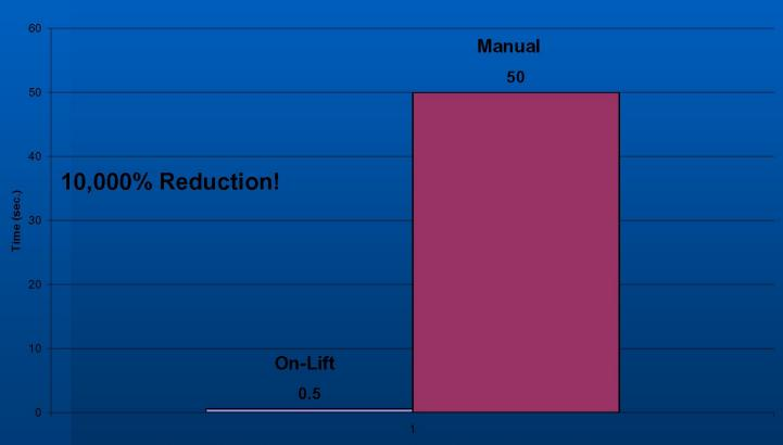
On-Lift eliminates manual effort of cranking landing gear.
