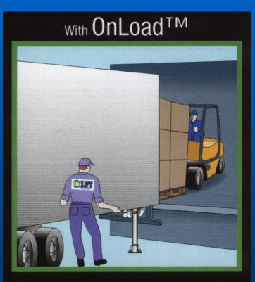
With OnLoad<sup>™</sup> delployed, rear end of trailer flush with dock allow forklift on and off freely
